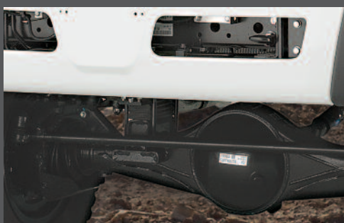
Full Floating Hypoid Type front axle and rear axles; front with Constant Velocity Universal Joints and rear with Positive Locking Limited Slip Differential.
