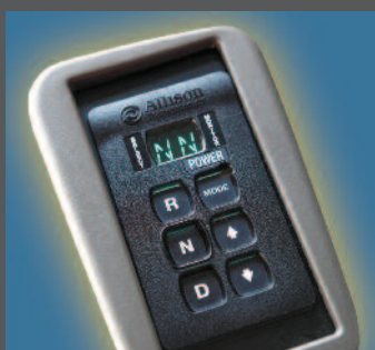
Allison 6 Speed Touch Pad Automatic Transmission with Generation 5 Control Systems for state of the art operation.
