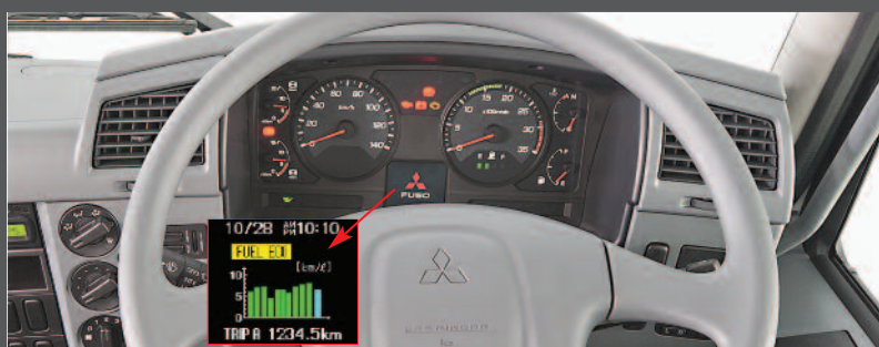
The new dash has a colour display that shows important information such as average and current fuel consumption.
