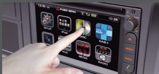
Every Fuso Heavy comes standard with the Fuso Multimedia Unit which includes satellite navigation with truck mapping, digital radio, Bluetooth® radio connectivity, iPod® interface and DVD player.
