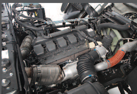
The new generation intercooled, turbocharged power plant provides 24% more torque and protects the environment with its SCR Emission Control.
