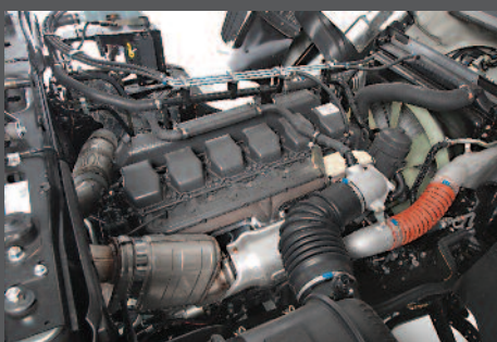
The new generation intercooled, turbocharged power plant provides 24% more torque and protects the environment with its SCR Emission Control.
